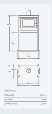
The raised firebox provides an uninterrupted view of the fire burning and allows usable space under the firebox. The slim nature allows the fireplace to be placed in almost any position taking up very little space. Placing a log into the fire has never been easier with no bending down required. A perfect feature and heater added simply to any home.
